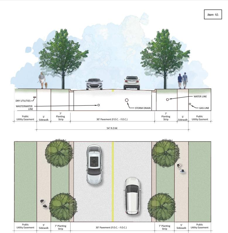
54' R.O.W. STREET TYPICAL SECTION  $_{\text{Scale: }1^{\prime\prime}=10^{\prime}}$
